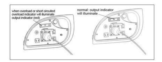
If the equipment is an inductive load, it will need more power for starting. Overload indicator and output indicator will turn on at the same time for a short period, that's normal. Red indicator turns off but green indicator still keeps on after equipment starts.
