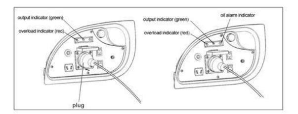
4. Turn on the equipment after output indicator (green) turns on If there is overload or malfunction in equipment, output indicator (green) will turn off and overload indicator (red) will turn on with no power output. TURN THE ENGINE OFF IMMEDIATELY and follow the instructions above.
