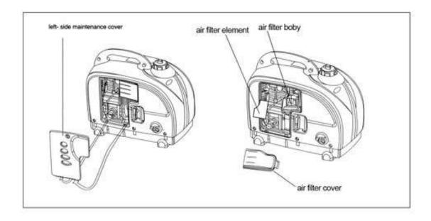
Never operate the engine without air filter. Rapid engine wear will result from contaminants, such as dust and dirt, being drawn through the carburetor into the engine.
