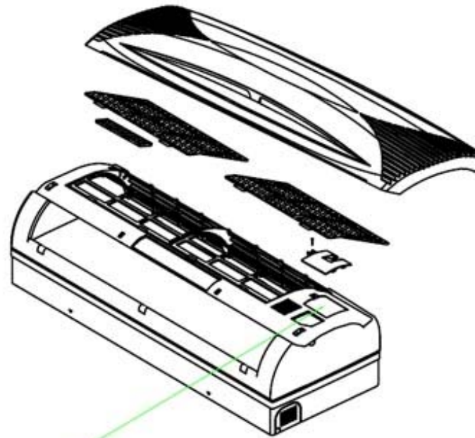
The wiring terminal of indoor unit
