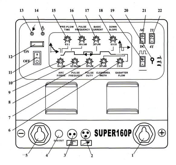
1, Output terminal to connect work piece;
