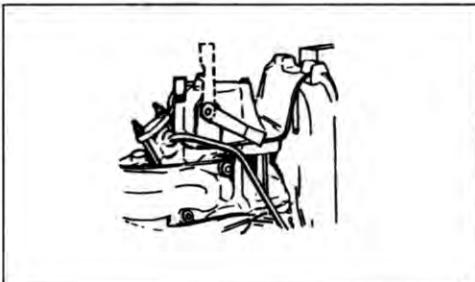
(3) Disassemble the rubber plug on the cover of rocker shaft and then fill about 2cc lubricant into it and return the plug to its position.
